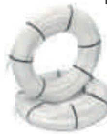
The **polipert** pipe is the only one without the internal aluminium layer, as it is completely made with plastic material. It includes 5 layers and the intermediate one is made of EVOH, whose function is to be an anti-oxygen barrier. Product low weight and the excellent flexibility allow an easy installation, even if it does not assure the same ductility of the products provided with the aluminium layer.
