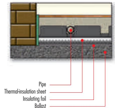
**NOTE:** wall-installation is also possible where a high energy supply is needed. Brackets and special components are available for the aforesaid type of application.
