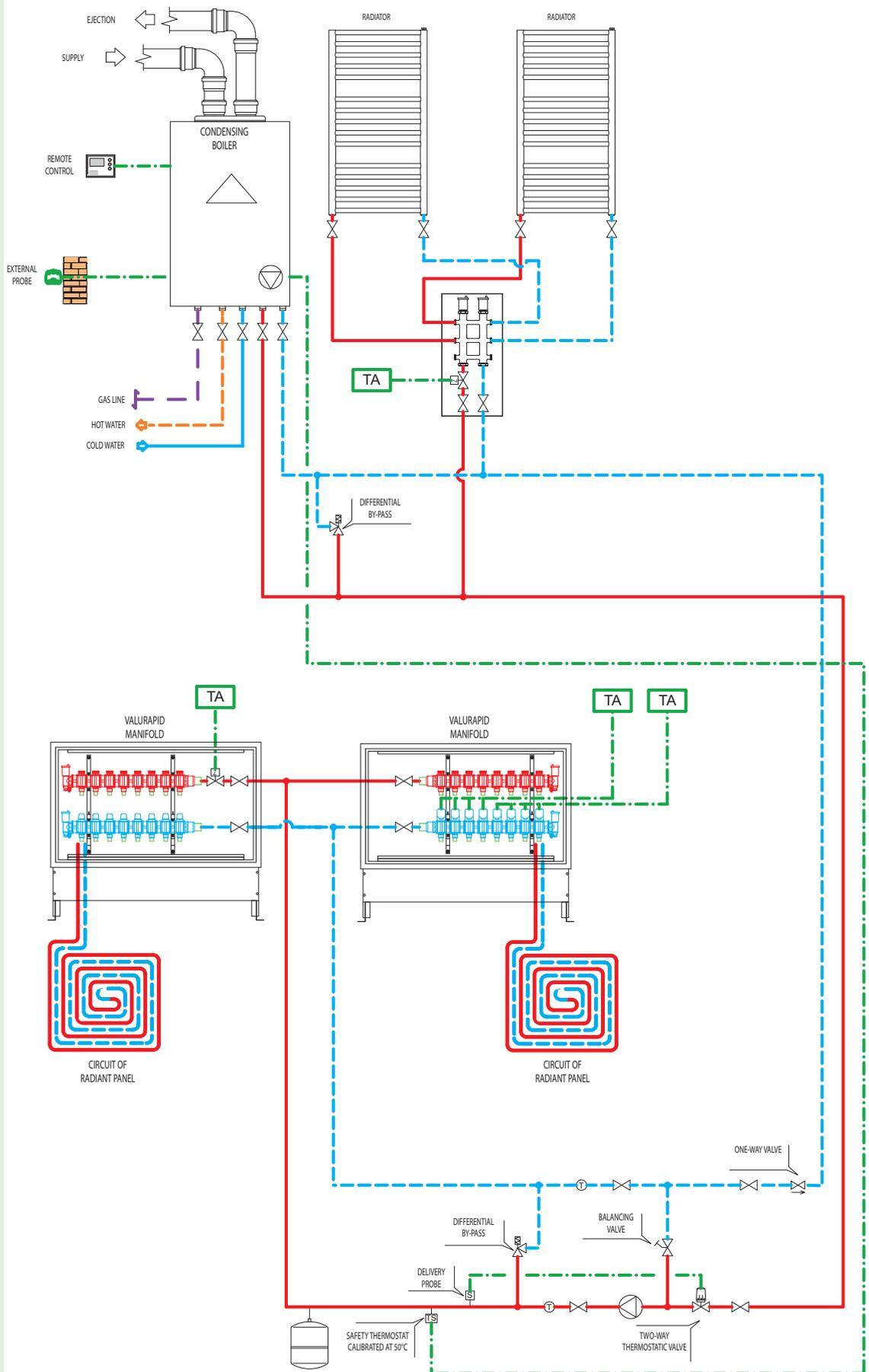
NOTE: DELIVERY TEMPERATURE ADJUSTMENT WITH SLIDING FIXED POINT BY MEANS OF CONDENSING BOILER
