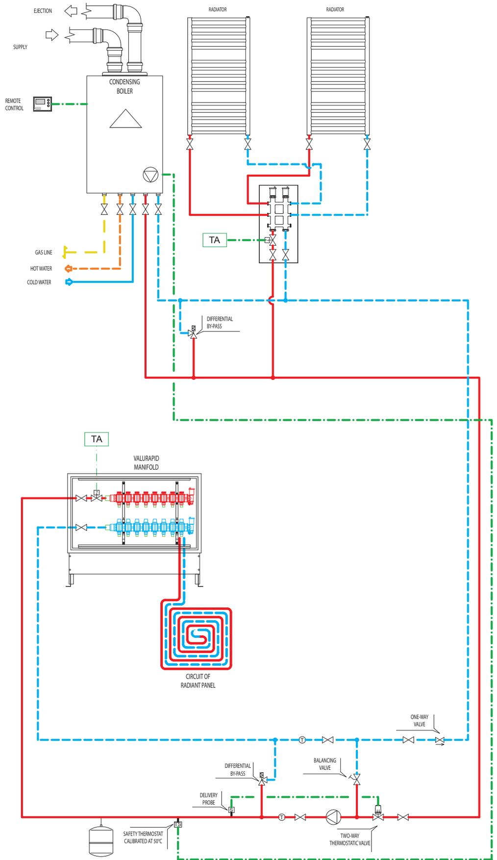
NOTE: DELIVERY TEMPERATURE ADJUSTMENT WITH FIXED POINT BY MEANS OF TWO-WAY THERMOSTATIC VALVE AND BALANCING VALVE
