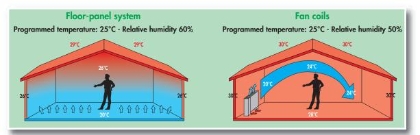
The floor-panel heating and cooling system is still the most comfortable climate-control system, which can offer an invaluable habitat and body wellness level.
